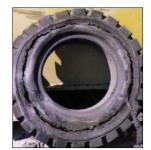
**CAUSE:** Excessive heat build up caused by overload or extreme distance, possible driver abuse in terms of exceeding maximum permissible speeds over sustained distances
