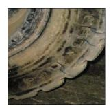
**CAUSE**: Tyre overload - At their capacity when fitted, any wear increases the load by volume, as the overloaded tyre wears it becomes smaller, therefore exacerbating the issue.
